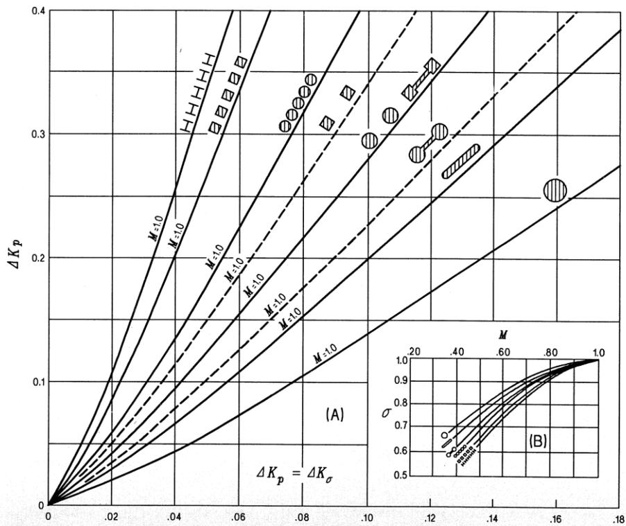
Figure 4 Incremental Backwater Coefficient for Piers (Hydraulics of Bridge and Waterways, 1978)
