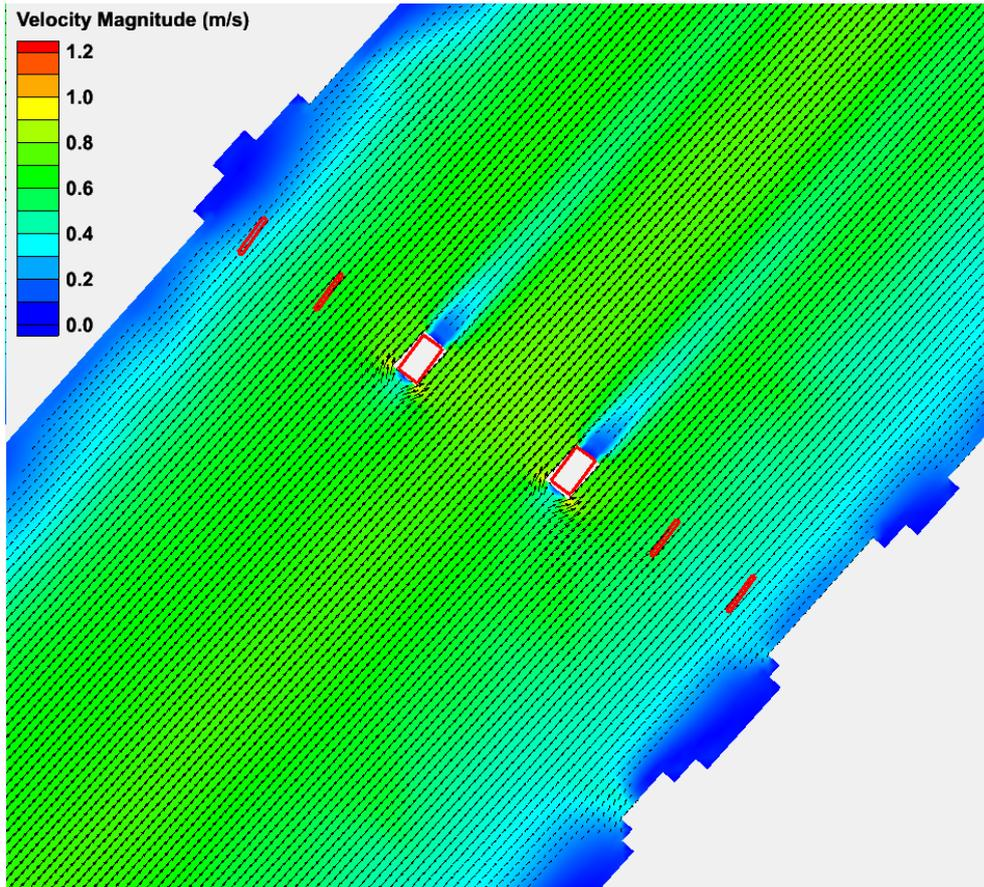
Figure 1 Velocity Magnitude and Direction; Piers Modelled by Modifying the Zpts
