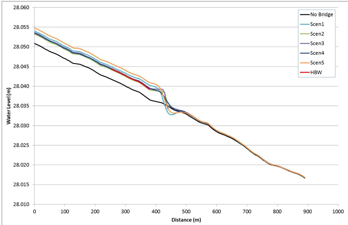
Figure 15 Water Surface Profiles; Bridge Modelling Methods
