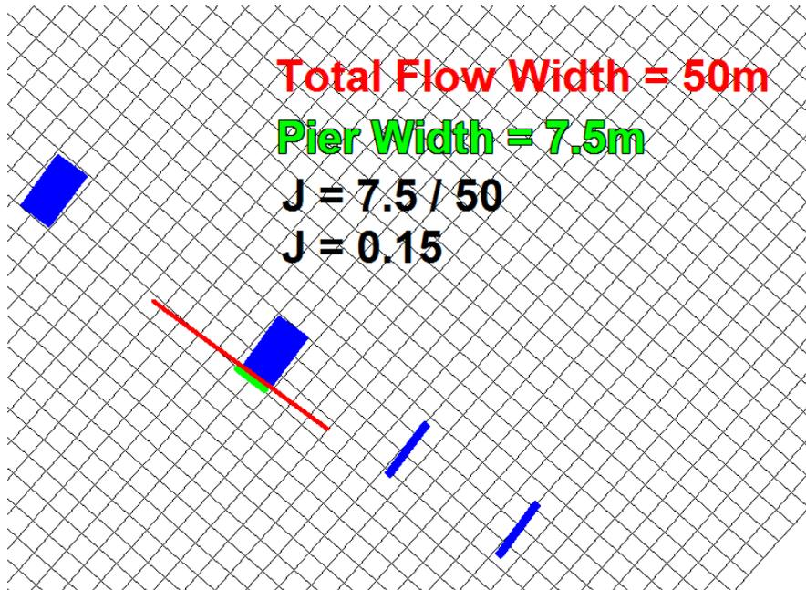
Figure 6 Blockage Calculation at Example Span
