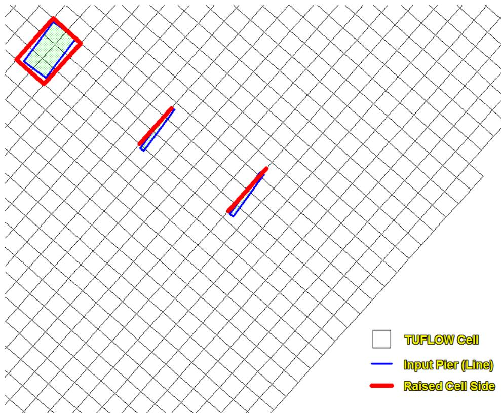
Figure 3 TUFLOW Cells and Pier Locations; 5m model
