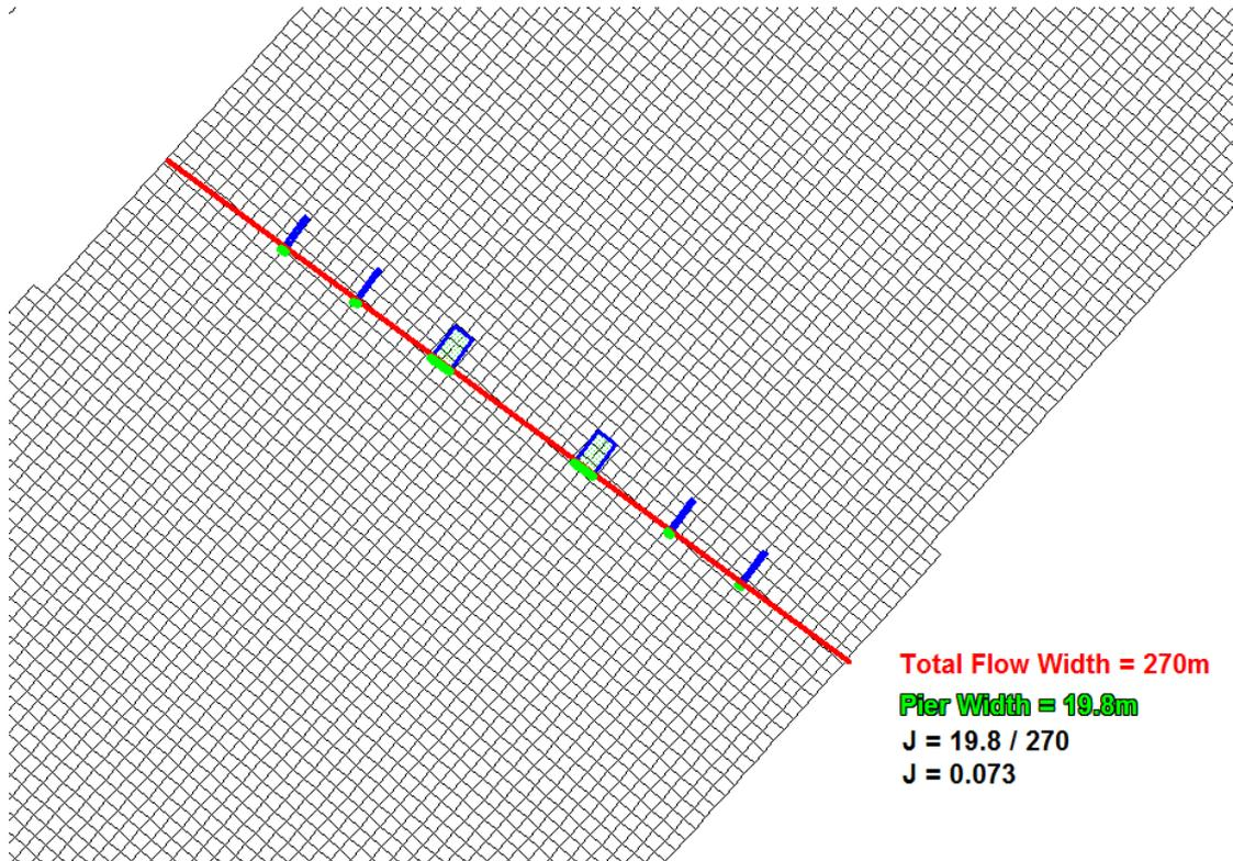
Figure 5 Blockage Calculation for Entire Bridge (Cell Size Independent)
