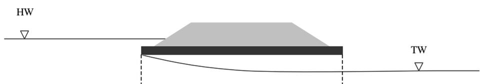
**Figure 1: Culvert Flow Control: Inlet control**
