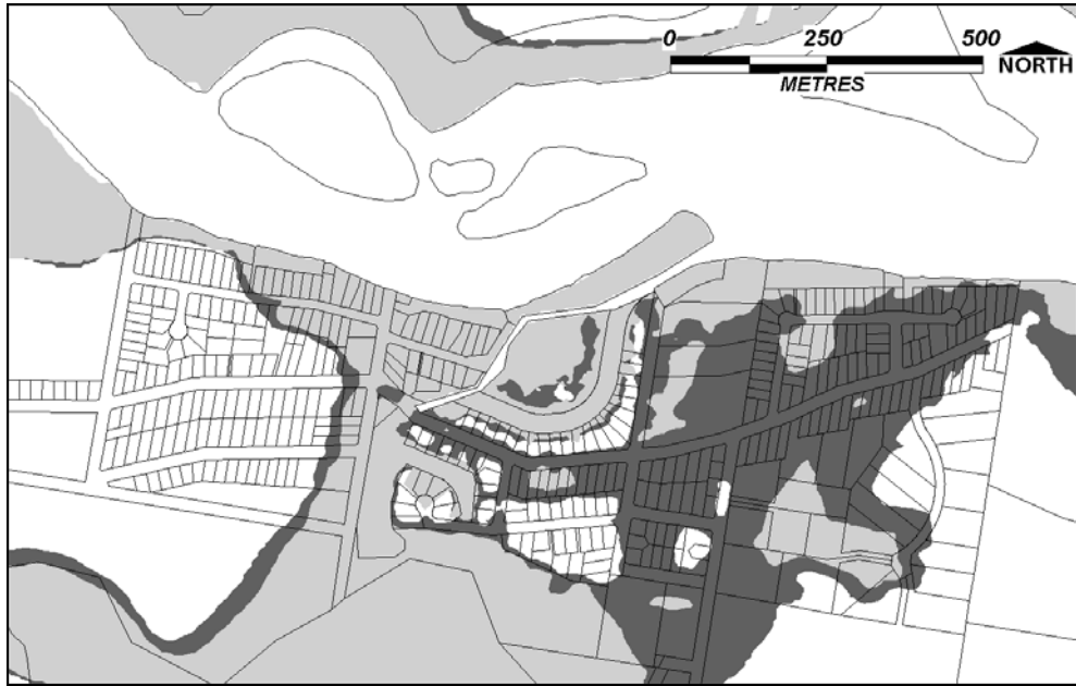
Figure 3 – Extent of Inundation (>0.5m deep) at Lake Conjola Township for Simulated Flood
