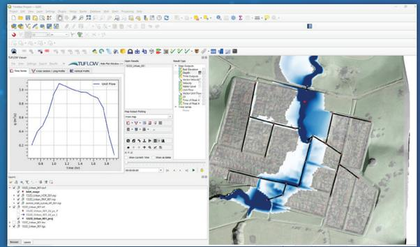
TUFLOW 1D and 2D solvers have been integrated for over 30 years, with continuous developments and enhancements making TUFLOW one of the most accurate and efficient hydraulic solvers available. Specific to integrated urban drainage, TUFLOW includes:
