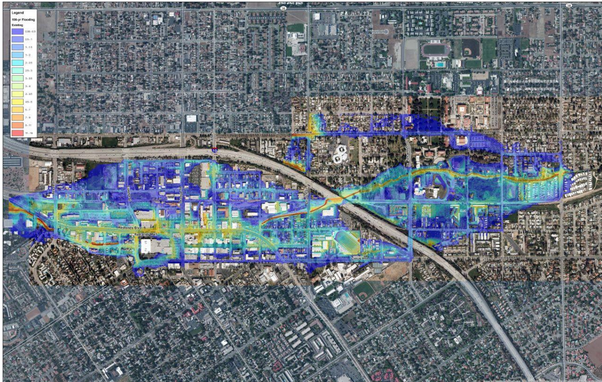
Figure 1: XPSWMM Urban Drainage 1D/2D Model – 100 Year Flood Inundation Depth
